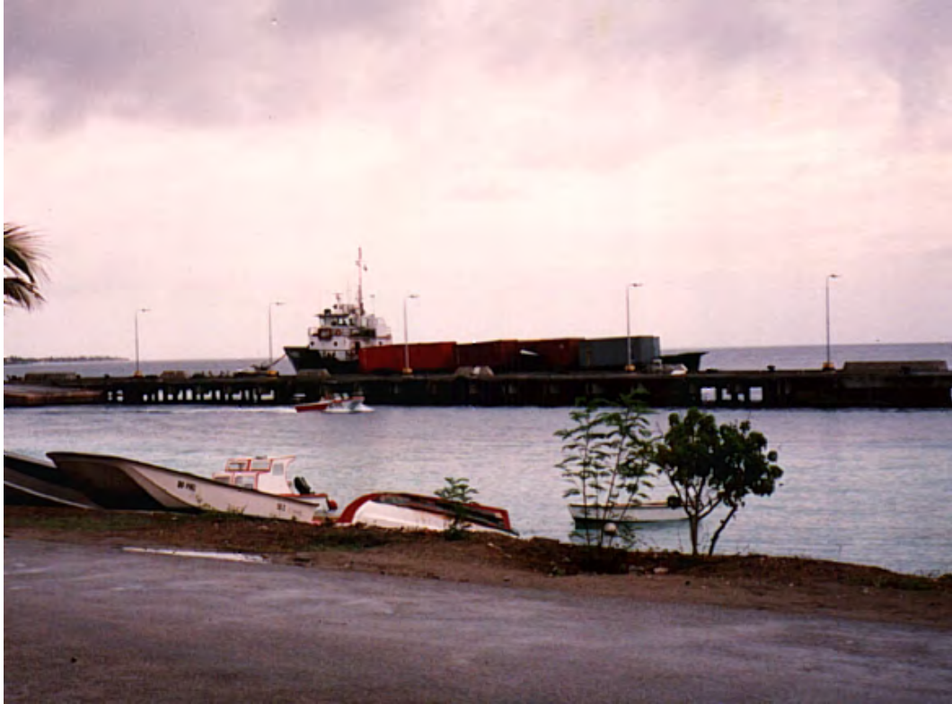
Figure 137: Inter-Island Shipping The Inter-island ship can carry eighteen 20' containers from Curacao to Bonaire.
