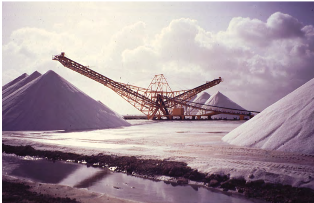
Figure 147: Mountains of Crystallized Salt The salt works in south Bonaire covers one-tenth of the island by area. Solar salt works can exist only in areas with ample sunshine, and evaporation that exceeds rainfall for most of the year.
