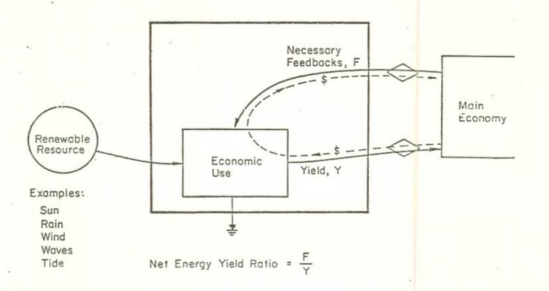
Figure 4. Diagram defining the net energy yield ratio for evaluating primary energy sources. Both F and Y should be in embodied energy units of the same quality. (a) nonrenewable source; (b) renewable resource.
