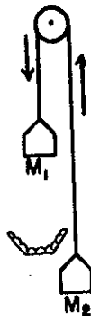
FIG. 1. Atwood's Machine. The power input due to the falling weight M_1 drives the elevation of weight M_2 which stores potential energy.
